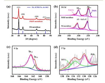
Fig. 3 (a) XRD patterns for PdSP metallene and Pd metallene. (b) Pd 3d XPS spectra for PdSP metallene and Pd metallene. (c) S 2p and (d) P 2p XPS spectra for PdSP metallene.
