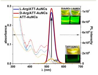
**Fig. 1** Absorption and emission spectra of ATT-AuNCs and two enantiomeric forms of Arg/ATT-AuNCs. Solid black arrow indicates PL enhancement of nanoclusters after addition of Arg to ATT-AuNCs. Photographs in the inset present eye-visible green luminescence.
