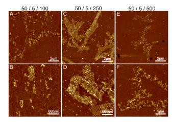
Fig. 3 The combined effect of Mg<sup>2+</sup>, Ni<sup>2+</sup> and Na<sup>+</sup> on lattice formation. (A and B), (C and D) and (E and F) show AFM images of different ST depositions when the concentrations  $C_{Mq^{2+}}/C_{Ni^{2+}}/C_{Na^+}$  are 50/5/100, 50/ 5/250 and 50/5/500 mM, respectively.
