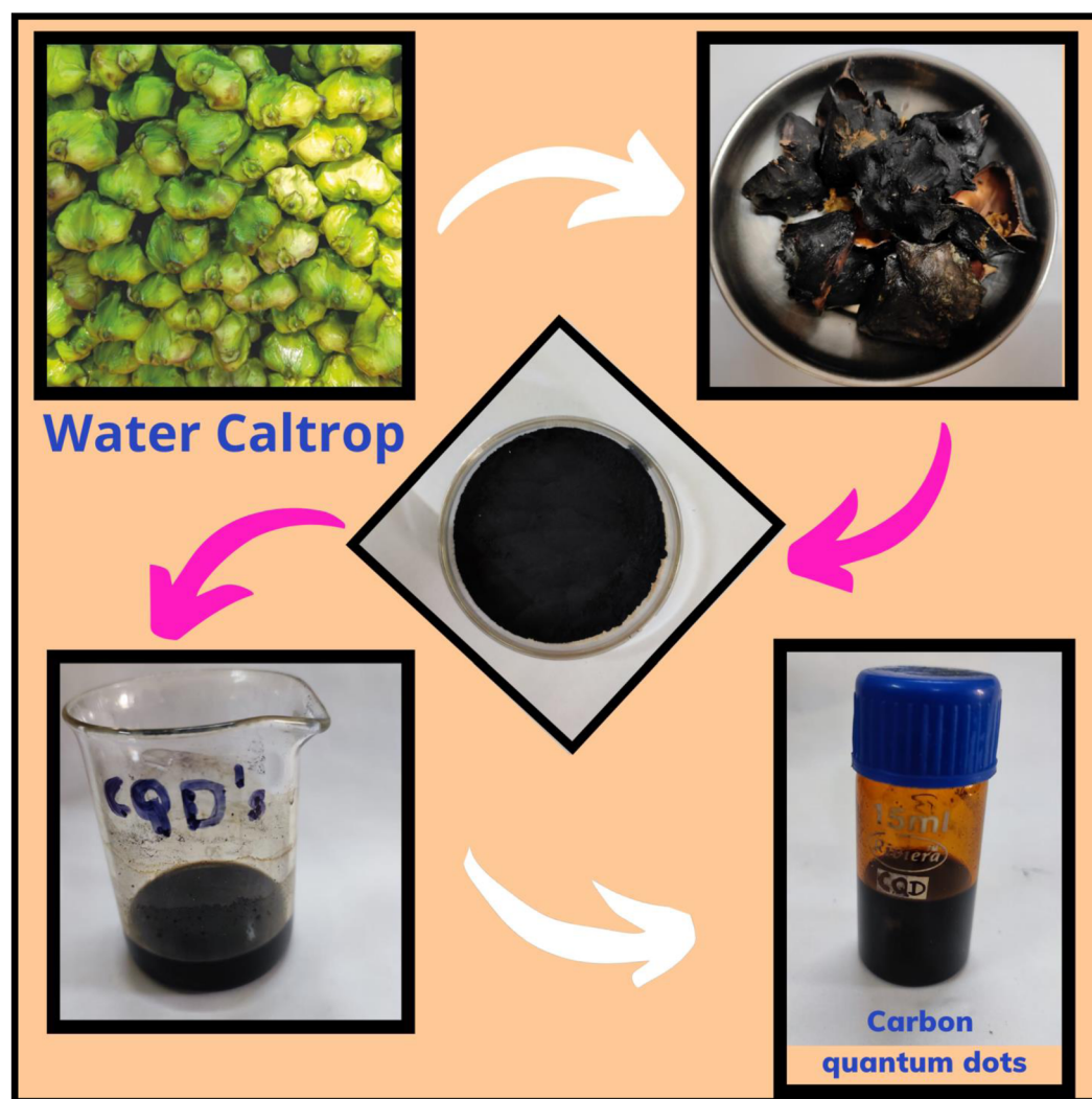
Scheme 1 The production process of carbon quantum dots from water caltrop peels.
