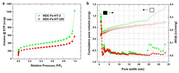
Fig. 3 (a) Isotherms of NDC-Fe-HT-X obtained from  $N_2$  sorption measurement. (b) The respective pore-size distribution from the adsorption branch employing the QSDFT model for slit and cylindrical pores.
