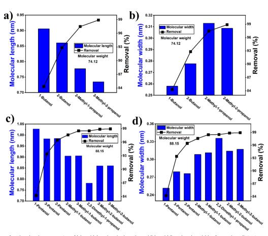
Correlation of molecular size parameter of (a) and (c) molecular length, and (b) and (d) molecular width of organic pollutant vs. removal rate (%) of reverse osmosis membrane. 308
