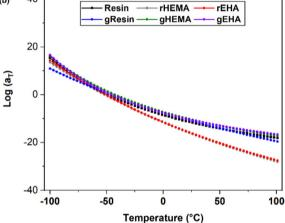
Fig. 8 (a) Mastercurves for printed neat and glass microsphere filled systems. (b) WLF shift factors for printed neat and glass microsphere filled systems fit to the WLF equation.
