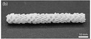
Additively manufactured complex composite structure. (a) Topdown view and (b) side view of an experimental mixing element with eight stages.
