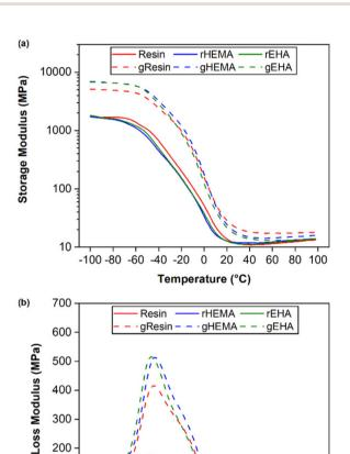
Fig. 6 DMA of printed specimens under single cantilever mode at 1 Hz. (a) storage modulus (E') and (b) loss modulus (E'')
