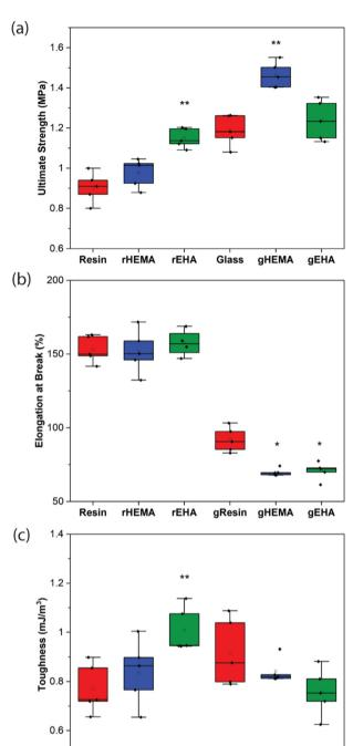
Fig. 4 (a) Ultimate strength, (b) elongation at break, and (c) toughness for neat and glass microsphere-filled samples. Individual data points as well as box and whisker plots are presented. \* indicates statistical differences from the control (either Resin or gResin). \*\* indicates statistical differences from all other conditions of the same type of sample (either neat or glass microsphere-filled)
