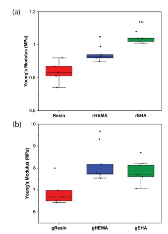
Fig. 3 Young's modulus values for (a) neat and (b) glass microspherefilled samples. Individual data points as well as box and whisker plots are presented. \* indicates statistical differences from the control (either Resin or gResin). \*\* indicates statistical differences from all other conditions of the same type of sample (either neat or glass microsphere-filled).
