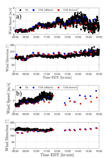
Fig. 8 Comparison plots showing differences between multirotor sUAS estimates of wind speed and wind direction at onshore (red) and offshore (blue) locations 10 m AGL on the (a) 5th and (b) 6th of August. The black markers correspond to the sonic anemometer (SA) observations collected 13 m AGL on August 5th and 6th.
