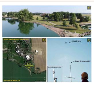
Fig. 3 (a) An aerial view showing the landscape surrounding the location where experiments were performed to validate multirotor sUAS wind estimates hovering next to a sonic anemometer installed 13 m AGL. (b) A satellite image of Wright State University Lake Campus, Ohio where multirotor sUAS and sonic anemometer wind comparisons were performed. (c) A close-up image showing the experiment setup used to validated multirotor wind estimates next to the sonic anemometer installed 13 m AGL.
