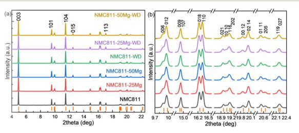
Fig. 6 SXRD patterns of the NCM811-based samples: (a) SXRD patterns with Bragg diffraction peaks from the R3m phase and (b) magnified view showing the peak splitting and asymmetric peaks due to the diffraction from doublets with a close interplanar distance.
