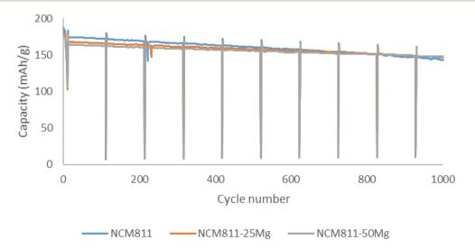
Pouch cell cycling of the unwashed NCM811 samples.
