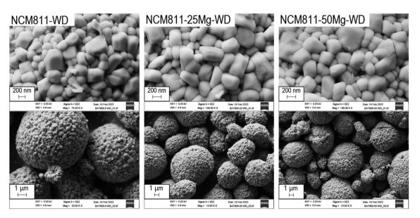
Fig. 5 Lithiated and washed NCM811, NCM811-25Mg and NCM811-50Mg samples.
