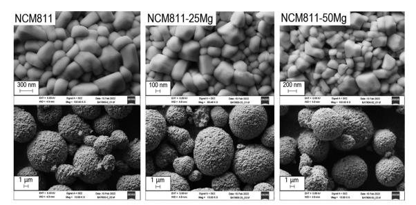
Fig. 4 Lithiated NCM811, NCM811-25Mg and NCM811-50Mg samples (unwashed).
