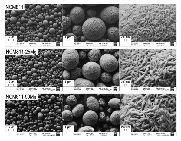
Fig. 2 Co-precipitated NCM811, NCM811-25Mg and NCM811-50Mg precursors.
