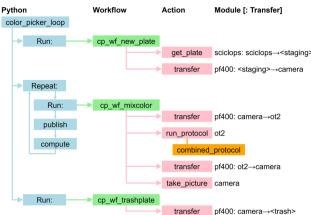
Fig. 11 The color-picker application. The Python code, color-picker\_app.py, implements logic that runs three distinct workflows, with the second (plus associated publish and compute steps) called repeatedly until termination criteria are satisfied. The orange box below the ot2 run\_protocol action gives the name of the protocol file. Module names are as in Table 2.
