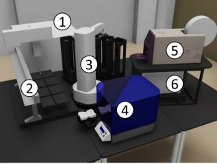
Fig. 6 The bio workcell, shown in real (left) and virtual (right) representations, comprises (1) liconic, (2) solo, (3) platecrane, (4) brooks\_peeler, (5) a4s sealer, and (6) hidex modules.
