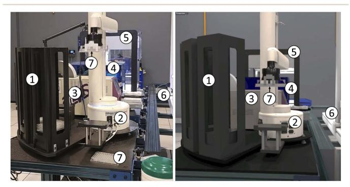
Fig. 10 Other views of the RPL workcell of Fig. 8, shown in real (left) and virtual (right) representations. Modules, from front to back: (1) plate stack; (2) sciclops stacker; (3) a4s\_sealer; (4) brooks\_peeler; (5) ot2; and (6) pf400. Also visible are (7) 96-well plates: one held by the sciclops in each image, and a second on the table in the real case.
