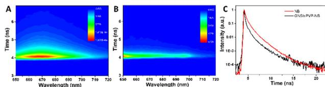
**Fig. 5** The TCSPC data carpets corresponding to NB in the absence (A) and the presence (B) of GNSts. The carpets present the intensity of the emission signal as a function of the emission wavelength and moment of time of photon arrival. The averaged kinetic traces (C) characteristic of each sample are also presented.
