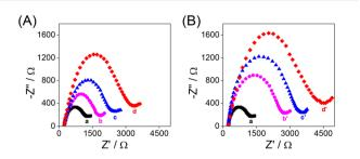
Fig. 1 Nyquist plots of different modified QCM Au chips in 5 mM [Fe  $(CN)_6 I^{3-/4-}$  (1:1) solution containing 0.1 M KCl (frequency,  $10^5-0.1$  Hz). (A) (a) Bare Au chip, (b) aptamer/Au chip, (c) BSA/aptamer/Au chip, and (d) RBD/BSA/aptamer/Au chip; (B) (a) bare Au chip, (b') antibody/Au chip, (c') BSA/antibody/Au chip, and (d') RBD/BSA/antibody/Au chip.  $C_{RBD}$  =
