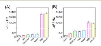
Fig. 4 Selectivity of the HF-QCM aptasensor (A) and immunosensor (B) for the RBD assay. RBD, 100 pg mL<sup>-1</sup>; interferent, 1 ng mL<sup>-1</sup>; the mixture contained the RBD (100 pg mL<sup>-1</sup>) and four interferents (each interferent, 1 ng mL<sup>-1</sup>).
