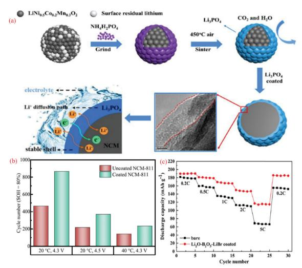
Fig. 7 (a) Schematic diagram of the experimental process.<sup>219</sup> (b) Achieved cycle numbers for different cycling conditions at an SOH of 80%. The calculation of the SOH is based on the capacity of the fifth cycle and (c) rate performance for uncoated NCM 523 and Li<sub>2</sub>O-B<sub>2</sub>O<sub>3</sub>-LiBr-coated NCM523. Reproduced with permission from Elsevier. 219
