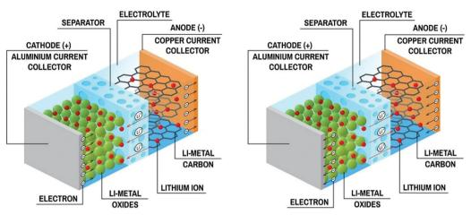
Fig. 3 Charge-discharge process in Li-ion battery (Image Credit: https://sivVector/Shutterstock.com).
