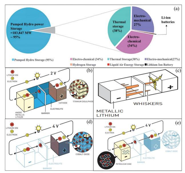
Fig. 2 (a) Contribution of worldwide energy storage projects to grid applications. 30 (b) Lithium-based battery using Li<sub>x</sub>TiS<sub>2</sub> as the cathode. (c) Formation of lithium whiskers/dendrites potentially leading to short-circuiting. (d) Lithium-based battery using  $\text{Li}_x \text{CoO}_2$  as the cathode. (e) Ion transfer cell lithiumion battery configuration. (© Johan Jarnestad/Royal Swedish Academy of Sciences 33).
