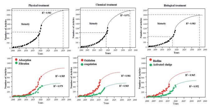
The S-curve analysis of different mining wastewater treatment methods and technologies as derived from the articles.
