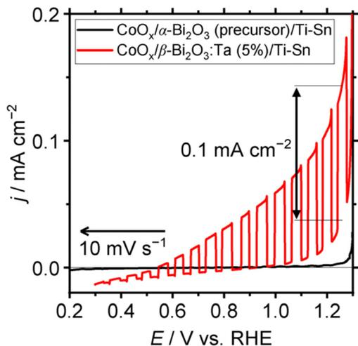
Fig. 10 LSV at  $10 \text{ mV s}^{-1}$  under light chops for  $\text{CoO}_x/\alpha\text{-Bi}_2\text{O}_3$  (precursor)/Ti-Sn and  $\text{CoO}_x/\beta\text{-Bi}_2\text{O}_3\text{:Ta (5\%/Ti-Sn}$  in 1 M potassium borate aqueous solution (pH 9). Sacrificial reagent: 0.1 M  $\text{Na}_2\text{SO}_3$ ; RE: Hg/Hg<sub>2</sub>Cl<sub>2</sub>/saturated KCl; CE: Pt wire; light source: Xe-lamp (MAX-303, 300 W) with cut-off filter (L42),  $>420 \text{ nm}$ ; temperature:  $25^\circ\text{C}$ .
