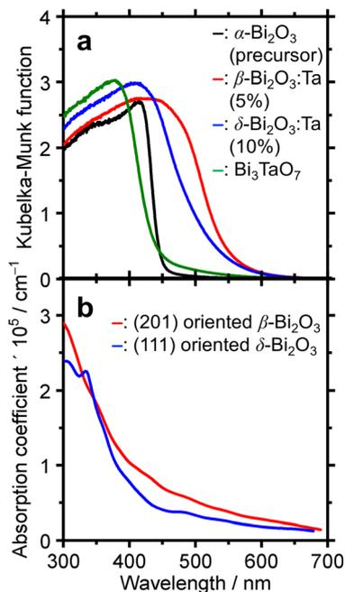
Fig. 7 (a) The DR-UV-vis spectra of  $\alpha$ -Bi<sub>2</sub>O<sub>3</sub> (precursor),  $\beta$ -Bi<sub>2</sub>O<sub>3</sub>:Ta (5%),  $\delta$ -Bi<sub>2</sub>O<sub>3</sub>:Ta (10%), and Bi<sub>3</sub>TaO<sub>7</sub>. (b) Simulated UV-visible optical absorption spectra of (201) oriented  $\beta$ -Bi<sub>2</sub>O<sub>3</sub> and (111) oriented  $\delta$ -Bi<sub>2</sub>O<sub>3</sub> slabs.
