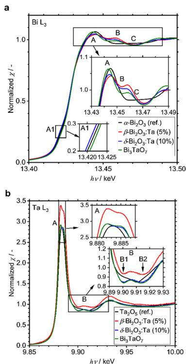
Fig. 4 (a) Comparison of the experimental Bi  $L_{3}$ -edge of  $\alpha$ - $\text{Bi}_2\text{O}_3$  (reference),  $\beta$ - $\text{Bi}_2\text{O}_3$ :Ta (5%),  $\delta$ - $\text{Bi}_2\text{O}_3$ :Ta (10%), and  $\text{Bi}_3\text{TaO}_7$ . (b) Ta  $L_{3}$ -edge XANES spectra of  $\text{Ta}_2\text{O}_5$  (reference),  $\beta$ - $\text{Bi}_2\text{O}_3$ :Ta (5%),  $\delta$ - $\text{Bi}_2\text{O}_3$ :Ta (10%), and  $\text{Bi}_3\text{TaO}_7$ .
