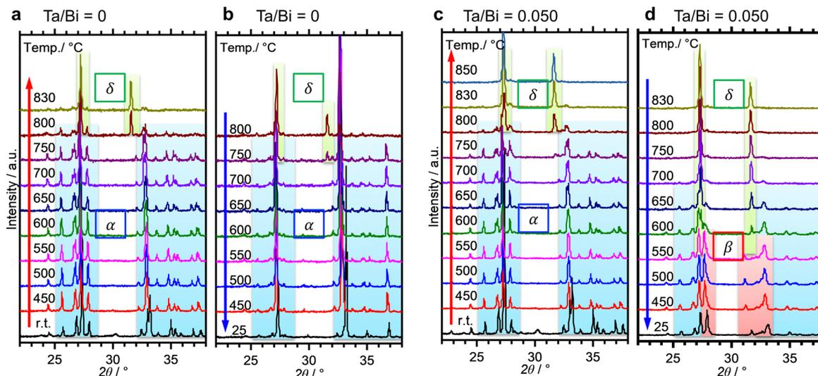
Fig. 2 *In situ* high-temperature XRD for the  $\text{Bi}_2\text{O}_3$  with Ta/Bi ratios of 0 (a and b) and 0.050 (c and d). The temperature was increased (a and c) and decreased (b and d) at the rate of  $10\text{ }^\circ\text{C min}^{-1}$  in static air. The assignments of the XRD peaks are indicated by coloring their backgrounds (blue:  $\alpha$  phase; red:  $\beta$  phase; green:  $\delta$  or cubic phase).
