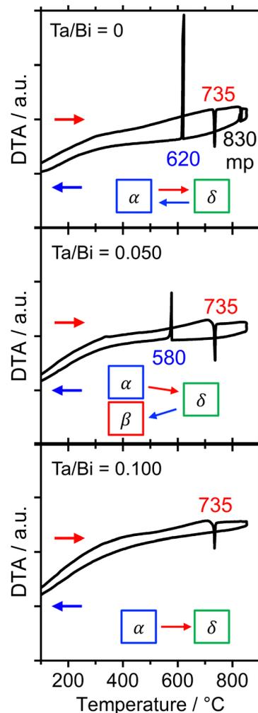
Fig. 1 DTA curves of the  $\text{Bi}_2\text{O}_3$  samples with Ta/Bi ratios of 0, 0.050, and 0.100. The temperature was increased and subsequently decreased at the rate of  $10 \text{ }^\circ\text{C min}^{-1}$  in flowing air.
