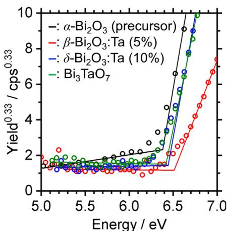
Fig. 8 Photoelectron spectra in air (PESA) of  $\alpha$ -Bi<sub>2</sub>O<sub>3</sub> (precursor),  $\beta$ -Bi<sub>2</sub>O<sub>3</sub>:Ta (5%),  $\delta$ -Bi<sub>2</sub>O<sub>3</sub>:Ta (10%), and Bi<sub>3</sub>TaO<sub>7</sub>.
