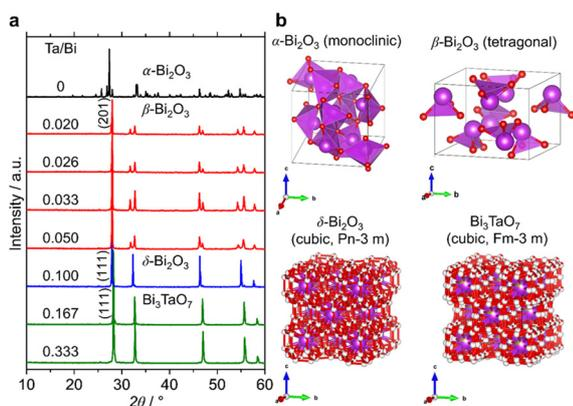
Fig. 3 (a) XRD patterns of the samples at the Ta/Bi ratio. (b) Schematics of the crystal structures from ICSD 94229 ( $\alpha$ - $\text{Bi}_2\text{O}_3$ ), 417638 ( $\beta$ - $\text{Bi}_2\text{O}_3$ ), 38436 ( $\delta$ - $\text{Bi}_2\text{O}_3$ ), and 161407 ( $\text{Bi}_3\text{TaO}_7$ ).
