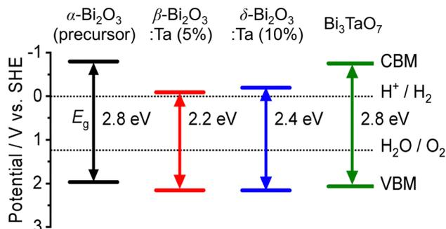
Fig. 9 The experimental band positions of  $\alpha$ -Bi<sub>2</sub>O<sub>3</sub> (precursor),  $\beta$ -Bi<sub>2</sub>O<sub>3</sub>:Ta (5%),  $\delta$ -Bi<sub>2</sub>O<sub>3</sub>:Ta (10%), and Bi<sub>3</sub>TaO<sub>7</sub>. The bandgap ( $E_g$ ) and valence band maximum (VBM) of each sample were determined by DR-UV-vis spectroscopy (Fig. 7a) and photoelectron spectroscopy in air (PESA) (Fig. 8), respectively.
