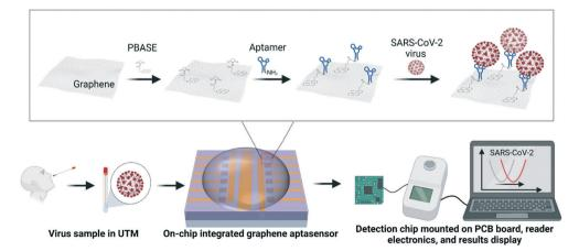
Fig. 1 Schematics of the SARS-CoV-2 virus detection using an on-chip integrated GFET aptasensor with portable electronics and the software presenting real-time detection results on a laptop. The zoomed-in area in the middle shows the schematics of the functionalization of the aptamer. The chip layout allows the different functionalization of two sections on a chip comprising 6 GFETs each.
