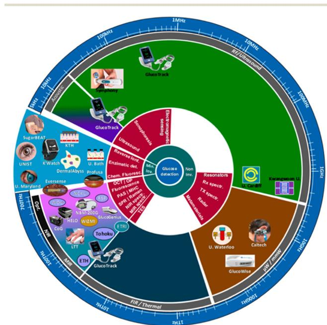
Fig. 13 Chart of current technologies and devices for CGM.<sup>16</sup> The frequency range corresponding to each technology is also displayed. Reproduced from ref. 16 with permission from MPDI, Copyrights 2019.
