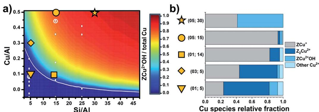
Fig. 4 (a) Predicted Cu site compositional phase diagram *versus* Si/Al and Cu/Al ratios. Color scale indicates predicted fraction of  $ZCu^{2+}OH$ . Adapted with permission from ref. 85. Copyright 2016 American Chemical Society. (b) Relative fractions of Cu species; the label “other  $Cu^{2+}$ ” refers to very minor contributions from residual, partially hydrated  $Cu^{2+}$  species. Unpublished figure reporting data from ref. 86.
