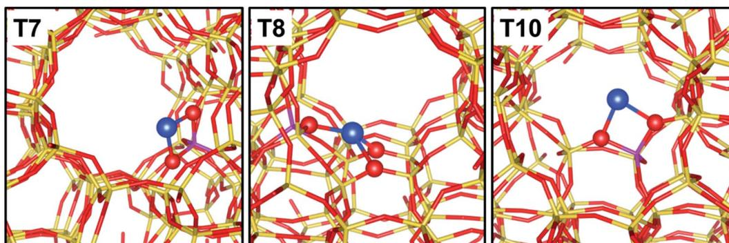
Fig. 3 Graphical representation of  $\text{Cu}^+$  sites balancing Al sitting in the T7, T8 and T10 crystallographic positions of ZSM-5. Colour code: blue, Cu; yellow, Si; magenta, Al; red, O. Unpublished figure, structural models obtained from DFT calculations as reported in ref. 37.
