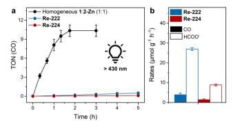
Fig. 3 Photocatalytic CO<sub>2</sub> reduction performance. (a) TON(CO) vs. time plot for MOF samples, including the homogeneous reference (black trace). (b) Product evolution rates averaged over the first two irradiation hours. Standard conditions: MOF sample (1.5 mg) suspended in MeCN (4 mL) and deionised H<sub>2</sub>O (0.12 mL) with BIH (225 mg), room temperature, continuous >430 nm irradiation.
