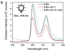
Fig. 5 Liquid-phase fluorescence spectra of MeCN/DMF (40/1 v/v) solutions containing 2-Zn (0.05 mM), 2-Zn (0.05 mM) and 1 (0.05 mM), and 2-Zn (0.05 mM) with the isolated  $Zr_6$ -oxo-node (0.2 mM). (a) Excitation at 415 nm. (b) Excitation at 515 nm.
