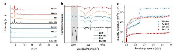
Fig. 2 Material characterisation for pristine and loaded PCN-222 and PCN-224 assemblies. (a) Measured PXRD data. (b) ATR-IR spectra including the reference for pure catalyst 1 (black trace) and with the characteristic region for Re(CO)<sub>3</sub> bands highlighted in grey. Full spectra in ESI.† (c)  $N_2$  sorption isotherms at 77 K.
