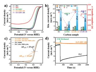
Fig. 6 (a) LSV curves of Pt/C, HPC and Fe/N–HPC, Fe/N–HPC-200 and Fe/N–HPC-400. (b) Electron transfer number,  $E_{1/2}$  and kinetic current density of Pt/C, Fe/N–HPC, Fe/N–HPC-200 and Fe/N–HPC-400. (c) LSV curves of Pt/C and Fe/N–HPC-200 before and after the accelerated durability test (ADT). (d) Chronoamperometric response of Pt/C and Fe/N–HPC-200 with 3 M methanol at 0.65 V and 1600 rpm. All data are obtained in  $O_2$ -saturated 0.1 M KOH electrolyte.
