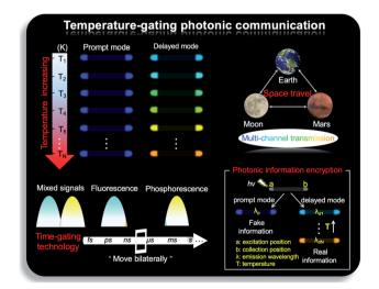
Fig. 7 Temperature-gating photonic communication. Diagram depicting the use of a 1D active waveguide microrod  $ZnCl_2$ –BZT in the field of temperature-gating photonic communications, which could transmit fluorescence and phosphorescence signals with different time and space domains over a large temperature span, enabling an improved density and high security of photonic communication.
