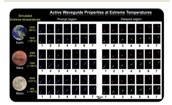
Fig. 6 Active waveguide properties at extreme temperatures. PL microscopy images of 1D microrod  $\rm ZnCl_2-BZT$  obtained by 375 nm laser excitation at different local positions under simulated extreme surface temperatures of (332 K and 183 K), Mars (308 K and 134 K), and the Moon (400 K and 90 K). Prompt regions: 420 nm–500 nm; delayed regions: 550 nm–600 nm (at high temperature), 500 nm–550 nm (at low temperature).
