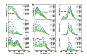
Fig. 4 Detecting the intermediate triplet excited states. Time-resolved emission spectra (TRES) of ZnCl<sub>2</sub>-BZT (a), ZnCl<sub>2</sub>-CBZT (b), and ZnBr<sub>2</sub>-BZT (c), which indicate that the energy of triplet excitons can be transferred from higher energy levels (400 nm-500 nm) to lower energy levels (500 nm-575 nm) through a rapid IC process which is followed by emission from the lowest triplet excited states.
