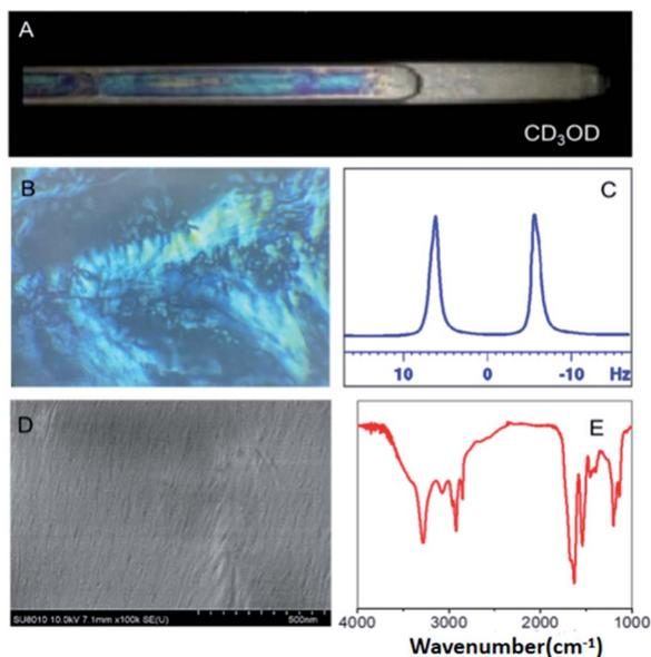
Fig. 1 (A) Photograph of the self-assembled OPA-1 (5%, w/v) in an NMR tube between two crossed polarizers. (B) POM images of OPA-1. (C) 1D  $^2\text{H}$  NMR spectrum ( $\text{CD}_3$ ) of the OPA-1 phase (5%, w/v). (D) SEM image of the aligned nanofibers at 5 wt%. (E) FT-IR spectrum of freeze-dried OPA-1 nanofibers.
