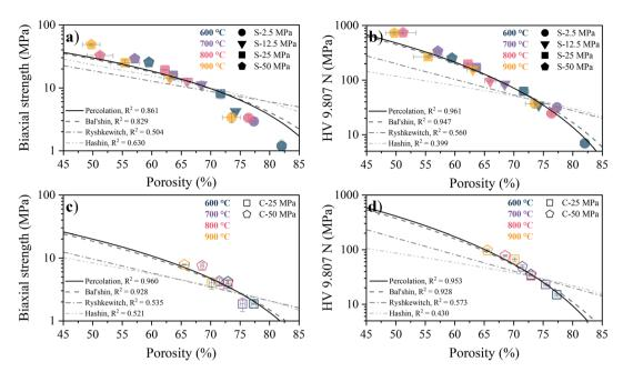
Fig. 9 Biaxial strength (a) and (c) and Vickers hardness HV 9.807 N (b) and (d) over porosity for varying sintering temperatures and pressures for S-and C-sintered COK-12 monoliths as well as corresponding Percolation, Bal'shin, Ryshkewitch, and Hashin fits.
