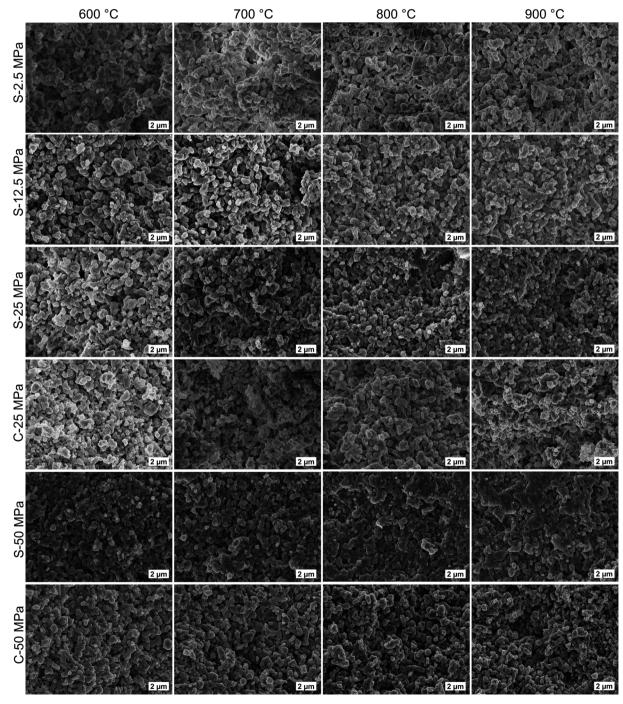
Fig. 7 SEM images of the fractured surfaces of S- and C-sintered COK-12 monoliths after mechanical testing
