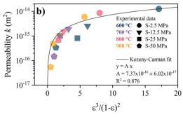
Fig. 11 Relation between porosity and pure water flow behavior for S-sintered monoliths. (a) water permeance  $L_p$  (b) permeability k and corresponding Kozeny–Carman fit.
