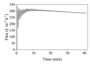
Fig. 12 Time-dependent flux during the filtration of surfactant-stabilized oil in water emulsion with 100 mg  $L^{-1}$  oil at a transmembrane pressure of 1 bar through an S-sintered monolith processed at 12.5 MPa and 800 °C. The initial COD of 366 mg  $L^{-1}$  could be reduced by 90% to 35 mg  $L^{-1}$ .
