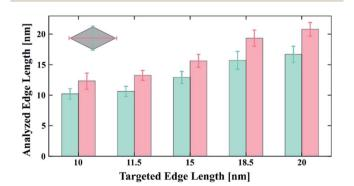
Fig. 3 Size distributions of LiYF<sub>4</sub>:Pr<sup>3+</sup> nanocrystals with 5% Pr<sup>3+</sup> concentration from 10 to 20 nm.
