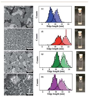
Fig. 2 TEM analysis of LiYF<sub>4</sub>: $Pr^{3+}$  nanocrystals with varying  $Pr^{3+}$  concentration: (a) 0.7, (b) 1.05, (c) 1.14, and (d) 1,47 at%. Corresponding particle size distributions (e–h) and photographs of colloidal dispersions in toluene (i–l).
