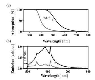
Fig. 1 Absorption (a) and emission (b) of strongly (black) and lightly (grey) colorized oleic acids.
