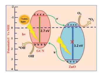
Fig. 26 Schematic depiction of the photocatalytic degradation mechanism of the ZnO/GCN heterojunction (reproduced from ref. 291 with permission from IOP Publishing)
