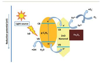
Fig. 27 Schematic depiction of the photocatalytic degradation mechanism of the g-C<sub>3</sub>N<sub>4</sub>/ZnO/Fe<sub>3</sub>O<sub>4</sub> heterojunction (reproduced from ref. 292 with permission from Elsevier).
