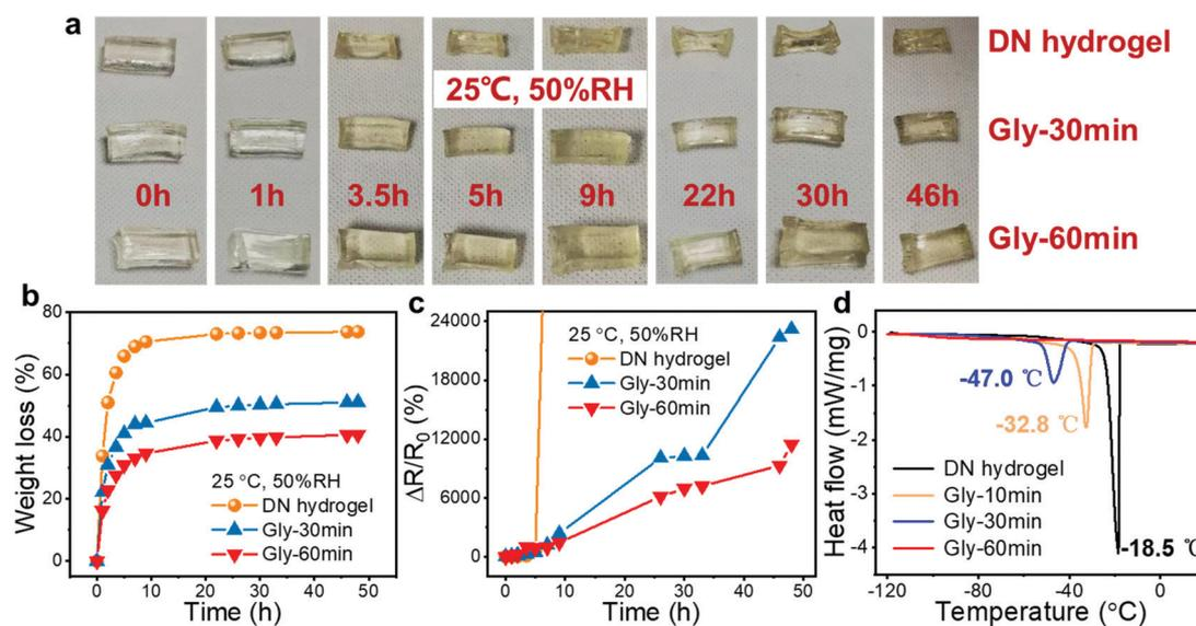
Fig. 3 (a) Optical images showing the morphology evolutions of the pristine hydrogel and organohydrogels obtained by soaking in Gly for 30 and 60 min when stored at  $25^\circ\text{C}$ , 50%RH for a series of time. (b) The relationship between weight loss percentage and time. (c) Curves showing the relative resistance variation versus time. (d) DSC spectra indicating the freezing points of the hydrogel and organohydrogels.
