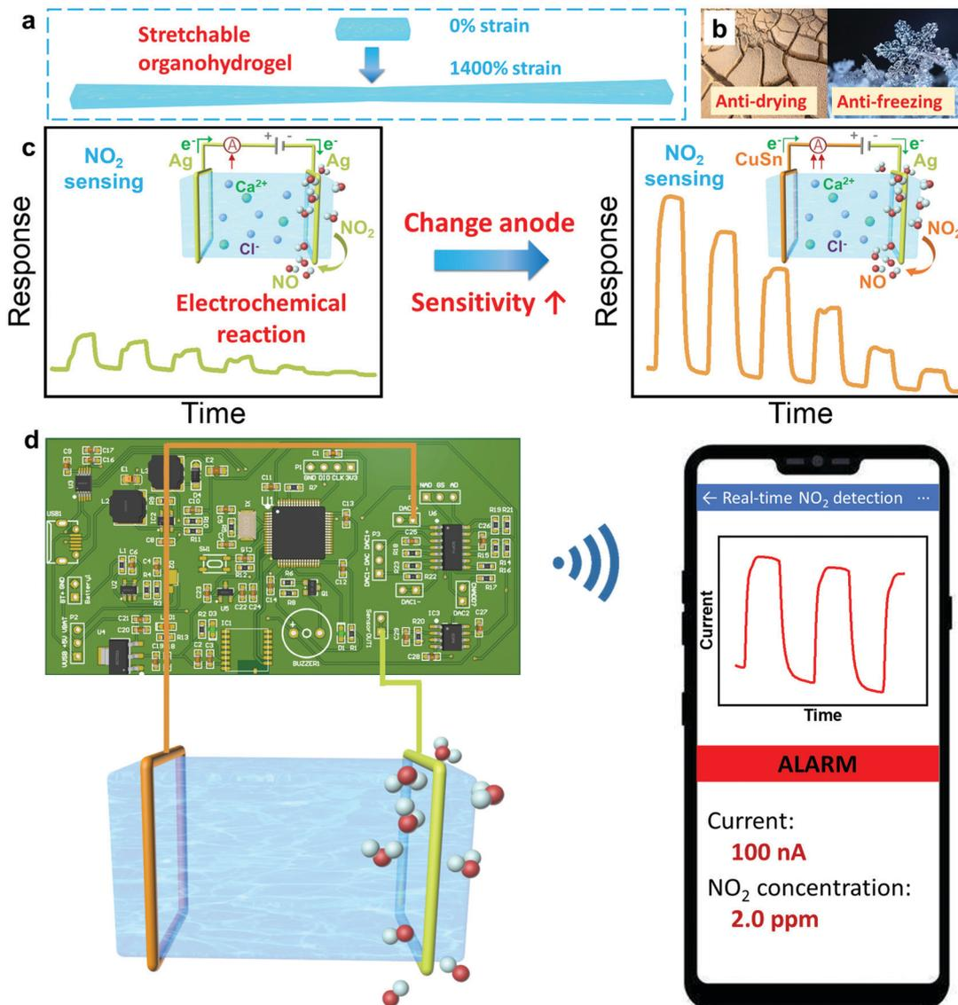
Fig. 1 Schematics illustrating (a) the high stretchability of the hydrogel, and (b) the anti-drying and anti-freezing capacities of the organohydrogels, respectively. (c) The electrode-dependent NO<sub>2</sub> sensing performance and sensing mechanism of the hydrogel sensors. (d) The wireless alarm demonstration of the hydrogel-based NO<sub>2</sub> sensor by a circuit board and an applet in a smartphone.
