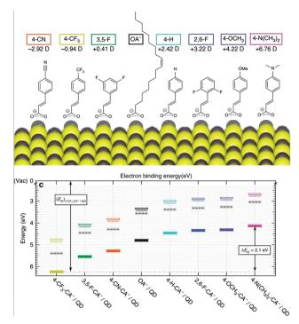
(Top) The molecular structures of organic molecules on PbS QDs and their dipole intensity; (bottom) the shifting of energy levels from the surface treatments with the dipole molecules determined by UPS. Reproduced with permission from ref. 31
