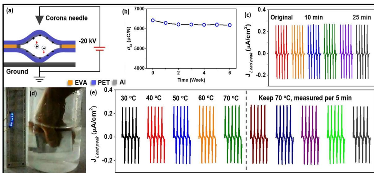
Fig. 23 Verification of PET/EVA PENG sample *via* (a) corona poling, and (b)  $d_{33}$  coefficient consistency over a six-week period; (c) stability of the generator under high moisture conditions; (d) illumination of six LEDs by pressing the device underwater; and (e) current output of the flexible PENG at high temperature (70 °C); reproduced with permission from ref. 309. Copyright 2017, Elsevier publication.
