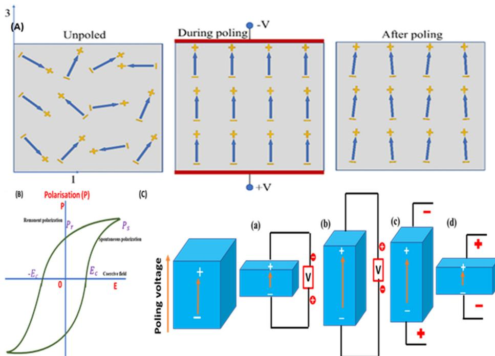
Fig. 2 (A) Domain alignment mechanisms before, during, and after the poling process; reproduced with consent from ref. 39. Copyright 2021, Springer Nature. (B) Polarisation–electric field hysteresis curve, and (C) piezoelectric material work as a sensor and actuator in various fields.
