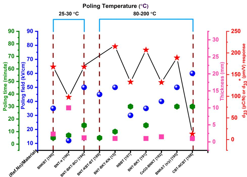
Fig. 12 Variation of  $d_{33}$  or  $d_{33}^*$  with the poling field, temperature, time and thickness.
