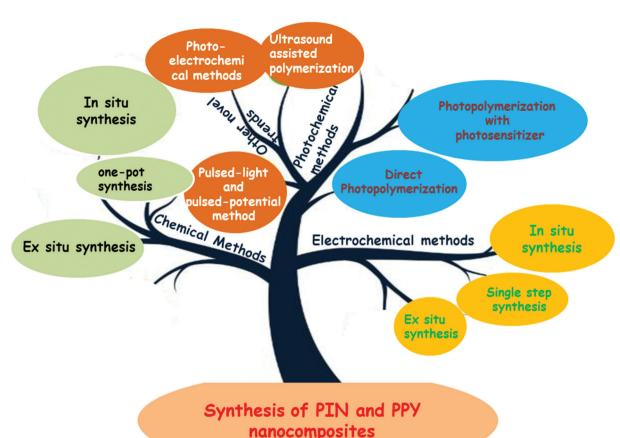
Graphical representation of the synthetic methods for PPY and PIN nanocomposites
