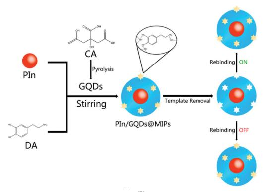
Fig. 7 Schematic of PIn/GQDs@MIPs synthesis. Reproduced with permission.<sup>276</sup> Copyright 2015, American Chemical Society
