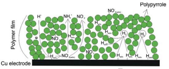
Fig. 6 An illustration of different reactions on the PPY-Cu electrode. Reproduced with permission.<sup>220</sup> Copyright 2015, Elsevier.
