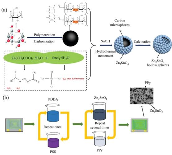
Fig. 3 Schematic representation of the synthesis of (a) Zn<sub>2</sub>SnO<sub>4</sub> hollow spheres and (b) PPy/Zn<sub>2</sub>SnO<sub>4</sub> nanocomposite film. Reproduced with permission. 134 Copyright 2018, Elsevier.
