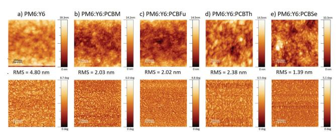
Fig. 5 AFM height (top) and phase (bottom) images of the blend films, (a) PM6:Y6; PCBM, (b) PM6:Y6; PCBM, (c) PM6:Y6; PCBFu, (d) PM6:Y6; PCBTh and (e) PM6:Y6; PCBSe. The scan size is  $1 \times 1 \mu m$ .
