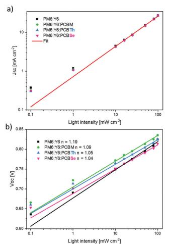
Fig. 3 (a)  $J_{SC}$  and (b)  $V_{OC}$  light dependence of binary OSCs and ternary OSCs with PCBM, PCBTh, and PCBSe
