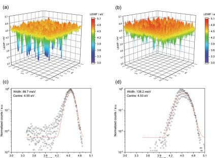
Fig. 8 LEWF maps showing the electronic terrain for (a) CZTSSe and (b) Ge5:CZTSSe after a 500 eV Ar<sup>+</sup> plasma etching treatment. Affiliated LEWF distribution showing the spread of points for (c) CZTSSe and (d) Ge5:CZTSSe.
