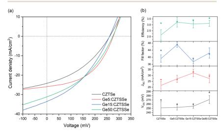
Fig. 6 CZTSSe device performance (a). J-V characteristics under a simulated AM1.5G spectrum and (b) statistical analysis of the performance parameters:  $V_{\rm OC}$ ,  $J_{\rm SC}$ , fill factor and conversion efficiency, showing the standard deviation.
