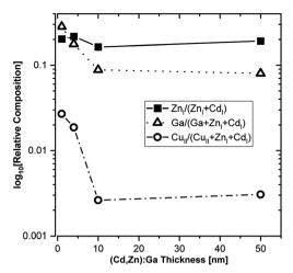
Fig. 6 HAXPES derived relative composition of the (Cd,Zn)S:Ga buffer layer as function of thickness. The elemental contributions with a numeral I and II subscript (e.g., Zn<sub>1</sub>) relate to different fit contributions to the evaluated photoemission lines (see Fig. 2-5): I and II refer to the main contribution (compound I) and to the secondary contribution (compound II), respectively. Ga has no subscript, as Ga 2p3/2 is fitted with one contribution (see Fig. S5†).
