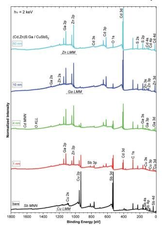
Fig. 1 HAXPES survey spectra recorded with 2 keV of the bare CuSbS<sub>2</sub> absorber (bottommost spectrum) and of the (Cd,Zn)S:Ga/CuSbS2 samples with buffer thicknesses varying from 1 nm (spectrum second from the bottom) to 50 nm (topmost spectrum). Vertical offsets were added for clarity.
