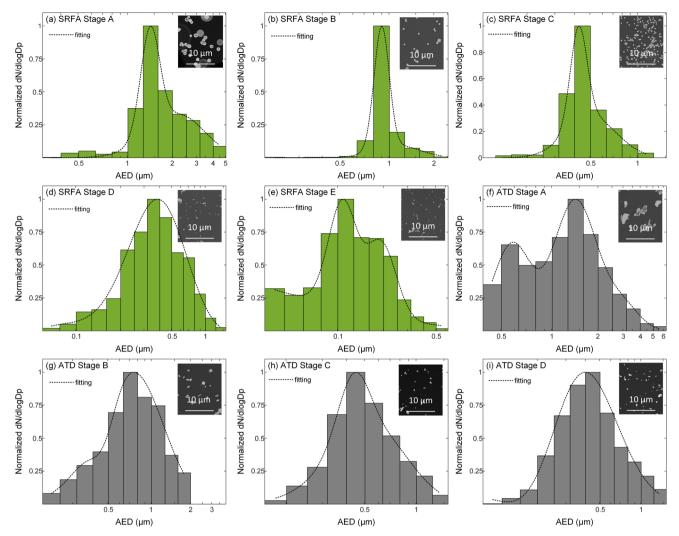
CCSEM-EDX measured particle size distribution of SRFA particles collected on stage A to E (a to e) and ATD particles collected on stage A to D (f to i). The insets are representative ESEM images of particles at each stage. AED stands for area equivalent diameter. The black dashed lines represent Gaussian fitting to the size distribution.
