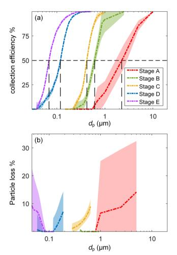
Fig. 2 (a) Particle collection efficiency at each stage as a function of particle diameter  $(d_p)$ . (b) Particle loss at each stage as a function of  $d_p$ . The shaded areas represent uncertainties in collection efficiency.
