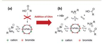
Fig. 13 Schematic representations of the dynamic surface stabilization of CsPbBr<sub>3</sub> NCs purified with acetone and dispersed in hexane (a) by oleylammonium bromide before the addition of excess OAm and (b) by oleylammonium bromide, oleylammonium oleate and OAm after the addition of excess OAm. The figure is modified with permission from ref. 33.
