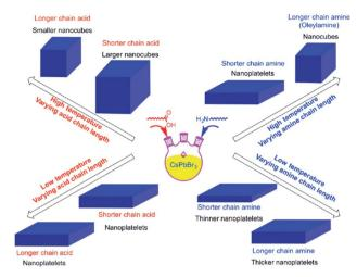
Fig. 8 Schematics illustrating the effect of temperature and type of ligand on the size and shape of NCs synthesized by the HI approach. The figure is reprinted with permission from ref. 141.
