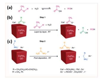
Fig. 18 Scheme showing (a) the ester hydrolysis to carboxylic acid and alcohol, (b) the anionic carboxylate ligand exchange and (c) cationic ligand exchange in CsPbl3 QD films. The figure is adapted with permission from ref. 207.
