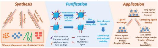
Fig. 20 A schematic showing the role of ligands during the synthesis, purification and application of perovskite NCs.
