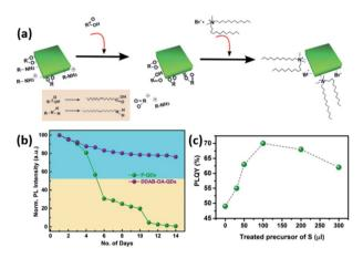
Fig. 16 (a) Illustration of the ligand exchange mechanism on  $CsPbBr_3$  QDs. (b) The variation of PL intensity with respect to time for unmodified QDs and DDAB-OA treated QDs. Both (a) and (b) are taken with permission from ref. 199. (c) The variation of PLQY values of  $CsPbBr_3$  QDs with the amount of the sulfide precursor added. This panel is taken with permission from ref. 200.
