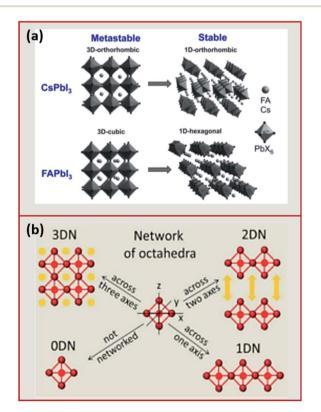
Fig. 2 (a) Illustration of the 3D to 1D phase transition in  $CsPbl_3$  and  $FAPbl_3$ . Reproduced with permission from ref. 27. (b) Schematic presenting the differences between the different dimensionalities (0DN, 1DN, 2DN and 3DN) depending on the connectivity of the octahedra. Reproduced with permission from ref. 56.
