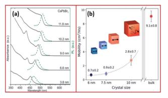
Fig. 4 (a) Absorption and emission of CsPbBr<sub>3</sub> NCs with variable size demonstrating quantum-size effects. (b) Size dependence of effective charge-carrier mobility of CsPbBr<sub>3</sub>. Panels (a) and (b) are reproduced with permission from ref. 57 and 81, respectively.
