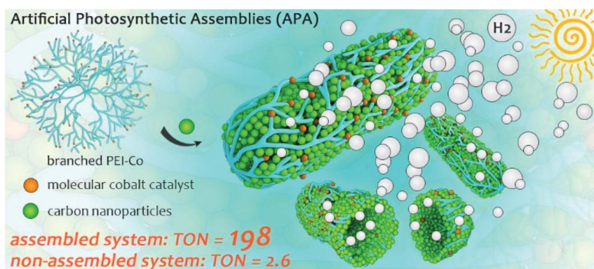
Scheme 15 Schematic diagram of photocatalytic H_2 production by the hollow-rod artificial photosynthetic assembly (APA) in water. Reproduced with permission from ref. 112. Copyright 2020, Royal Society of Chemistry.
