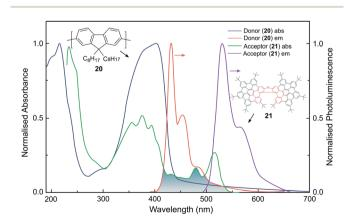
Fig. 13 The normalised absorption and photoluminescence ( $\lambda_{\rm ex}$ : 385 nm) spectra of thin films of the donor (20, thickness, t=140 nm) and acceptor (21, t=90 nm) systems used to achieve FRET. The overlap between the donor emission and acceptor absorption is shaded. This figure has been generated from the data present in the ref. 84.
