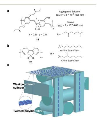
Fig. 12 (a) Structure of a poly(p-phenylene vinylene) (PPV) polymer used to achieve CP electroluminescence (EL).<sup>69</sup> (b) Structure of achiral and chiral polyfluorene (PF) polymers. (c) A representation of the proposed double twist cylinder blue phase.<sup>31</sup>
