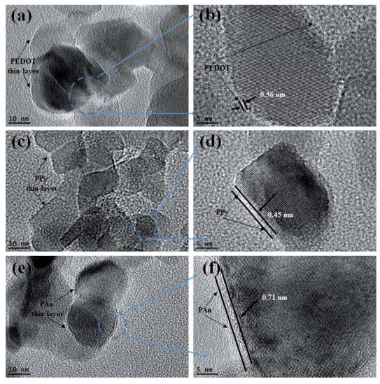
Fig. 5 HRTEM images of (a, b) TiO<sub>2</sub>@2PEDOT, (c, d) TiO<sub>2</sub>@2PPy, and (e, f) TiO<sub>2</sub>@5PAn composites.
