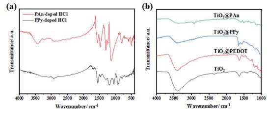
Fig. 3 FTIR spectra of (a) PAn-doped HCl and PPy-doped HCl, and of (b) bare-TiO<sub>2</sub>, TiO<sub>2</sub>@PEDOT, TiO<sub>2</sub>@PPy, and TiO<sub>2</sub>@PAn composites.
