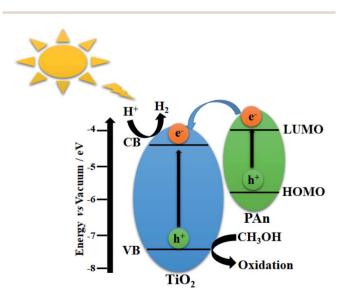
Fig. 16 Scheme illustrating the photocatalytic hydrogen production  $\it via$  water splitting over TiO<sub>2</sub>@PAn heterostructure.
