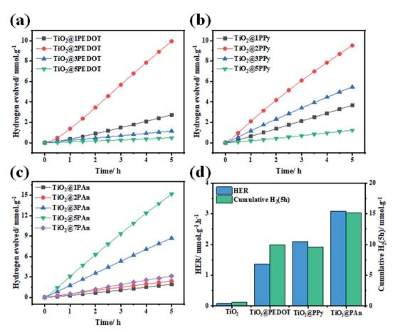
Fig. 10 Time course of  $H_2$  evolution over 50 mg of different weight percent of (a) poly(3,4-ethylenedioxythiophene) (b) polypyrrole (c) polyaniline relative to  $TiO_2$  (P25) in a 20% vol. aqueous methanol under UV light irradiation for 5 h (d) Histograms of optimum samples.
