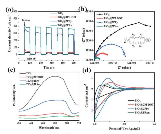
Fig. 13 (a) Transient photocurrent response (I-t) curves; (b) EIS Nyquist plots; (c) the photoluminescence spectra (PL) measured at an excitation wavelength of 350 nm and (d) cyclic voltammetry curves of TiO<sub>2</sub>, TiO<sub>2</sub>@2PEDOT, TiO<sub>2</sub>@2PPy, and TiO<sub>2</sub>@5PAn, photocatalysts.
