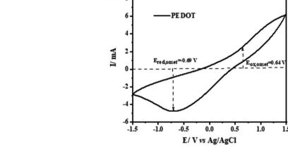
Fig. 14 (a-c) Cyclic voltammetry (CV) curves of pure PAn, PPy and PEDOT conducting polymers electrodes.
