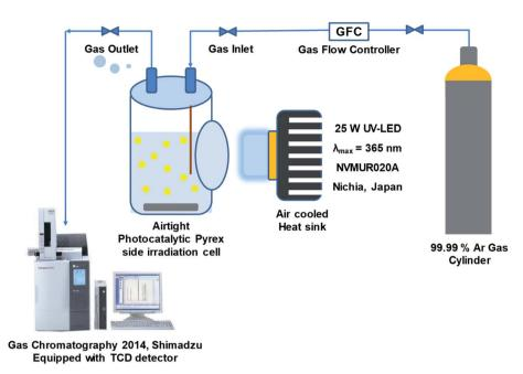
Fig. 2 Photocatalytic hydrogen production flow system.
