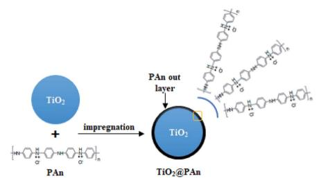
Fig. 1 Schematic illustration of TiO<sub>2</sub>@PAn composite fabrication.
