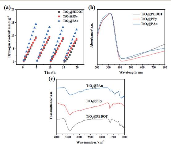
Fig. 11 (a) Cyclic photocatalytic hydrogen generation over 50 mg of TiO<sub>2</sub>@PEDOT, TiO<sub>2</sub>@PPy, and TiO<sub>2</sub>@PAn in 20% (vol.) methanol aqueous solutions under UV light illumination ( $\lambda = 365$  nm), (b) DRS, and (c) FTIR spectra TiO<sub>2</sub>@2PEDOT, TiO<sub>2</sub>@2PPy, and TiO<sub>2</sub>@5PAn composites after 20 h of light irradiation.
