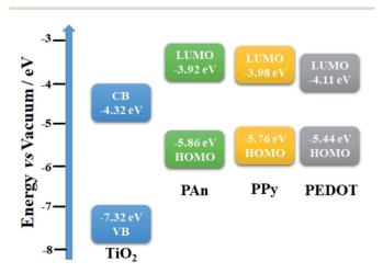
Fig. 15 Energy band structure of TiO2@PEDOT, TiO2@PPy, and TiO2@PAn photocatalysts.
