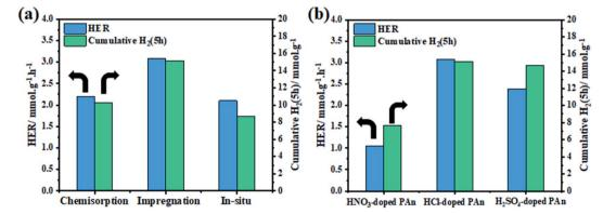
Fig. 9 The initial and cumulative (5 h) hydrogen evolution rate of (a)  $TiO_2$ @5PAn composites fabricated by chemisorption, in situ polymerization, and impregnation methods and (b) TiO<sub>2</sub>@5PAn composites modified with various counterions, NO<sub>3</sub><sup>-</sup>, SO<sub>4</sub><sup>2-</sup>, and Cl<sup>-</sup>.
