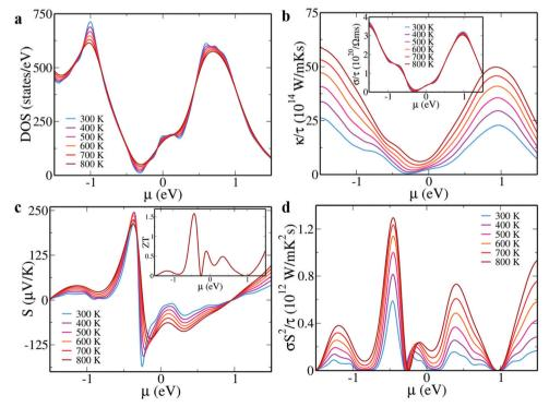
Fig. 3 (a) DOS; (b) thermal conductivity (inset: electrical conductivity); (c) Seebeck co-efficient (inset: ZT@800 K) and (d) power factor of Sn<sub>10</sub>Pb<sub>5</sub>BiTe<sub>16</sub> as a function of chemical potential ( $\mu$ ) at various temperatures. The conductivity and power factor values are reported by scaling it with  $\tau$ .
