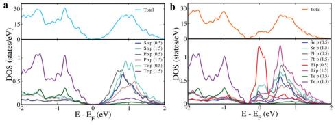
Fig. 2 pDOS of (a)  $Sn_{11}Pb_5Te_{16}$ ; and (b)  $Sn_{10}Pb_5BiTe_{16}$ . The energy levels are shifted with respect to the Fermi level of the configurations, which is set to zero.
