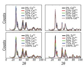
Fig. 2 X-ray diffraction pattern obtained for the nanoparticles based on our 864 cation model in 500 ps molecular dynamics at 300 K starting from the 0 K geometry. The simulation aims to capture the signature with a Cu X-ray source ( $\lambda$  = 1.541838 Å).
