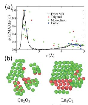
Fig. 3 (a) Comparative plot for partial  $Ce^{3+}-O^{2-}$  g(r) for our final  $Ce_2O_3$  nanoparticles obtained from molecular dynamics. The points indicated in the plot are the position and intensities for the pure infinite crystal in three different phases. (b) Visualization of low strain cations obtained for our final  $Ce_2O_3$  and  $La_2O_3$  models, using OVITO. 51 The atoms shown as green are classified as cubic crystal atoms, while the red ones are trigonal.
