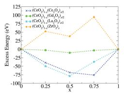
Fig. 6 Excess energy ( $E_{\rm exc}$ ) calculated from the structures at zero temparature.
