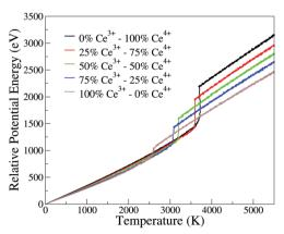
Fig. 5 Potential energy of the nanoparticle (relative to the 0 K configuration) as a function of instantaneous temperature for the CeO<sub>2</sub>–Ce<sub>2</sub>O<sub>7</sub> 864 cation nanoparticles. Analogous plots for all systems are provided as ESI.†
