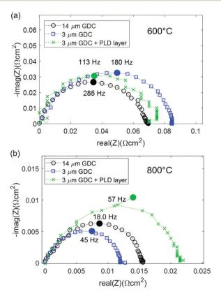
Fig. 4 (a) Impedance spectra of different GDC anodes at (a) 600 °C and (b) 800 °C. The high frequency offset was subtracted from all spectra for the sake of easier comparability
