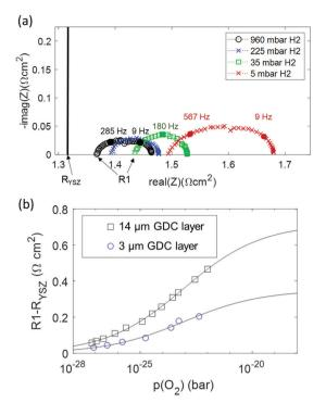
Fig. 6 (a) Impedance spectra of a symmetrical GDC 3  $\mu$ m |PtGDC|Pt cell at 600 °C in 25 mbar H<sub>2</sub>O, and varying H<sub>2</sub> partial pressures. The black vertical line in part (a) represents the "real" electrolyte resistance  $R_{YSZ}$ . (b) Difference of offset resistance ( $R_1$ ) and real electrolyte resistance ( $R_{YSZ}$ ) as a function of  $p(O_2)$ . The solid line represents the fit according to eqn (2).
