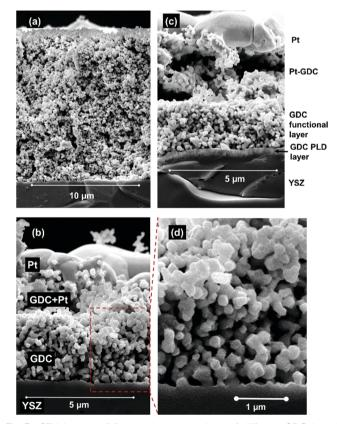
Fig. 3 SEM images of fractured cross-sections of different GDC-based electrodes after electrochemical measurements. (a) Brushed GDC layer with 14 µm thickness - the Pt current collector delaminated during fracturing. (b) Spin-coated, 3 µm thick GDC layer with Pt-GDC|Pt current collector. (c) Spin-coated GDC layer with PLD-grown GDC film at the electrode/electrolyte interface and Pt-GDC|Pt current collector on top. (d) Magnification of the functional layer in (c).
