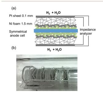
Fig. 2 (a) Sketch of mounting and contacting of a symmetrical GDC anode cell with porous Pt current collecting layer. (b) Photograph of the cell measurement assembly. Four symmetrical model cells are mounted in the single chamber impedance test rig and measured in one run by a multiplexed measurement
