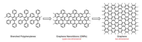
Scheme 1 From branched polyphenylenes to GNRs and infinite graphene sheets.
