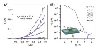
Fig. 13 (A)  $I_d - V_d$  characteristics of the 9-AGNR FET. (B)  $I_d - V_g$  of the device showing high  $I_{\rm on}$  > 1  $\mu A$  for a 0.95 nm wide 9-AGNR and a high  $I_{\rm on}/I_{\rm off}$  of  $\sim 10^{5.197}$  Copyright 2017. Adapted with permission from Macmillan Publishers Ltd: Nature Communications.
