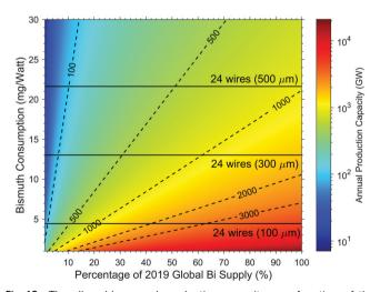
Fig. 12 The allowable annual production capacity as a function of the percentage of global Bi supply based on 2019 and the bismuth consumption per cell. The wafer size is assumed to be 210  $\times$  210 mm<sup>2</sup>.
