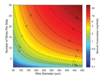
Fig. 13 Calculated bismuth consumption as a function of the number of wires per side and the wire diameter assuming a 3  $\mu$ m coating of SnBi and cell efficiency of 25.11%.
