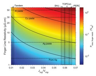
**Fig. 9** Relative finger resistance losses with different ratio of  $J_{\rm mp}/V_{\rm mp}$  and line resistivity of fingers. The same metallization pattern (1 mm finger spacing with 12 busbars) is assumed for all data points. Solid contour lines represent relative power losses from finger series resistance.
