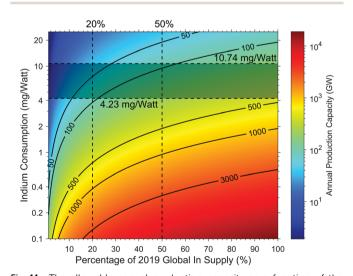
Fig. 11 The allowable annual production capacity as a function of the percentage of 2019 global Indium supply and the Indium consumption (mg  $W^{-1}$ ) per cell in typical SHJ solar cells. The assumed cell efficiency is 25.11% with an area of 210  $\times$  210  $\text{mm}^2$ . Shaded regions represent the range of indium consumption in current SHJ solar cells shown in Table 7.
