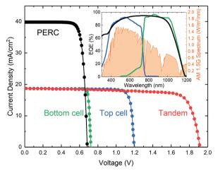
**Fig. 8** JV curves and external quantum efficiencies (EQE) of a typical 21.9% efficient industrial PERC solar cell (black), a 28.1% efficient two-junction two-terminal Si-based tandem solar cell<sup>73</sup> (red), the top (blue) and the bottom cell (green) of the same tandem device.
