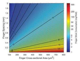
**Fig. 3** Finger silver consumption for 23.8% efficient PERC cells as a function of front finger spacing and finger cross-sectional area. The wafer area is assumed to be 210  $\times$  210  $\text{mm}^2$ . The hashed region has the finger silver consumption above the 2 mg W $^{-1}$  target. Contour lines represent different finger silver consumption levels.
