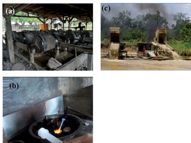
Fig. 1 Details of the measurement sites. (a) Ball mill method in Poboya near Palu, (b) Mercury-gold amalgam is heated, evaporating the mercury and leaving gold at a gold shop, (c) dredging operation in the Kahayan River.
