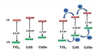
Fig. 13 Relative energy levels in TiO<sub>2</sub> photoelectrode co-sensitized with CdS and CdSe NPs. Reproduced with permission from ref. 118.
