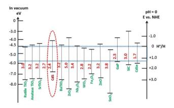
Fig. 2 The band gap positions for CdS and other SCs relative to the redox potential of water.
