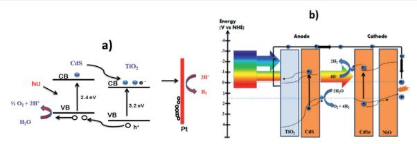
Fig. 12 Photoelectrochemical water splitting. (a) Mechanism of PEC water splitting by  $CdS-TiO_2$  nanocomposite. Reproduced with permission from ref. 225 (b) photoelectrolysis cell consisting of CdS coupled  $TiO_2$  photoanode and CdSe coupled NiO photocathode. Reproduced with permission from ref. 227.
