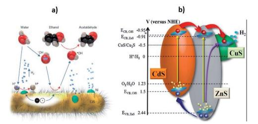
Fig. 15 (a) The proposed hole shuttle mechanism for H<sub>2</sub> generation over the cysteine-stabilized CdS nanorods. The hydroxyl anions scavenge the holes and carry away the positive charges which in turn oxidize the ethanol to acetaldehyde. The blue arrow represents the movement of species and red arrows denote a redox reaction. Reprinted with permission from ref. 78. (b) Charge transfer illustration in ZnS-CuS-CdS photocatalyst. Reprinted with permission from ref. 303.
