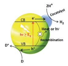
Fig. 7 Cocatalyst triggered photocatalytic process where D and D<sup>+</sup> represent an electron donor and its oxidized form respectively. Reproduced with permission from ref. 160.
