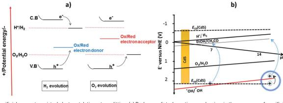
Fig. 16 Sacrificial reagents assisted photocatalytic water splitting. (a) Redox mediated reaction mechanism in the presence of sacrificial reagents. Reproduced with permission from ref. 307 and (b) the band edge position of CdS (CB and VB) and the relative redox potential of water, hydroxyl anion, and ethanol oxidation. Reproduced with permission from ref. 78.
