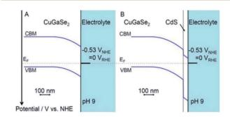
Fig. 11 Band alignment at interfaces for (A) CuGSe<sub>2</sub> and (B) CdS/CuGSe<sub>2</sub> electrodes. Reprinted with permission from ref. 209.
