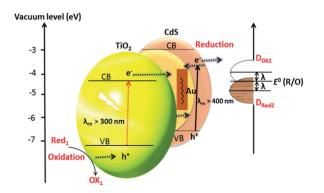
Fig. 14 Schematic energy diagram for the Z-scheme electron transfer mechanism. Energy band illustration of CdS–Au–TiO<sub>2</sub> system where  $E^0$  (R/O) is the standard electrode potential of MV<sup>+</sup>/MV<sup>2+</sup> and D<sub>Red2</sub> and D<sub>Ox2</sub> illustrate the occupied and unoccupied states, respectively. *I* represent the reorganization energy. Reproduced with permission from ref. 250.
