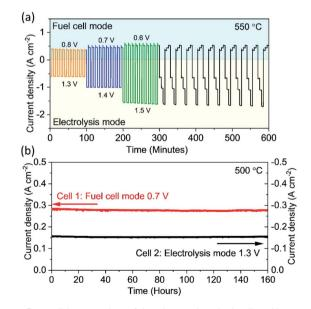
Fig. 5 Reversible operation of the electrochemical cell and long-term stability in fuel cell and electrolysis modes. (a) Reversible operation between the electrolysis and fuel cell mode at 550 °C when the cell working voltage is transiently changed; and (b) long-term stability testing of the cell in fuel cell mode at 0.7 V and in electrolysis mode at 1.3 V and 500 °C.
