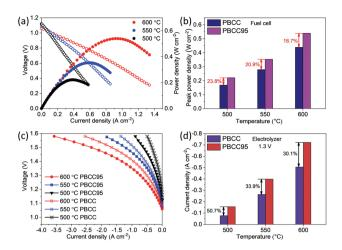
Fig. 4 Electrochemical performances of PBCC95 and PBCC electrodes at 500, 550, and 600 °C. (a) I-V and current-power density (I-P) curves of PBCC95 in fuel cell mode; (b) peak power density comparison between PBCC95 and PBCC; (c) I-V curve of PBCC95 and PBCC electrodes in electrolysis mode; (d) electrolysis current density comparison of PBCC95 and PBCC at 1.3 V.
