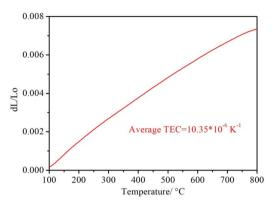
Fig. 7 The thermal expansion coefficient of PrBaNiMn over the temperature range of  $100-800\,^{\circ}\text{C}$ .
