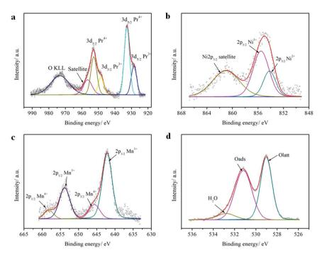
Fig. 4 (a) Pr 3d; (b) Ni 2p; (c) Mn 2p and (d) O 1s core level XPS spectra of PrBaNiMn powder.
