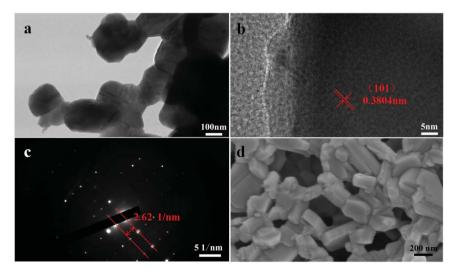
Fig. 3 (a) Bright-field TEM of PrBaNiMn powder; (b) the high-resolution TEM (HRTEM) images of PrBaNiMn at the (101) lattice plane; (c) the FFT of the (101) lattice plane; (d) the SEM image of PrBaNiMn.
