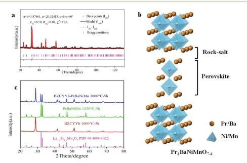
Fig. 2 (a) Rietveld refinement plot of PrBaNiMn powder using X-ray powder diffraction data,  $R_{wp}$  and  $\chi^2$  represent the weighted profile factor and reduced chi-square; (b) the crystal structure of Pr<sub>2</sub>BaNiMnO<sub>7- $\delta$ </sub>; (c) XRD patterns of PrBaNiMn, BZCYYb fired at 1250, 1000 °C and the dry-mixed composite powder BZCYYb-PrBaNiMn (5 : 5) fired at 1000 °C for 5 h, respectively.
