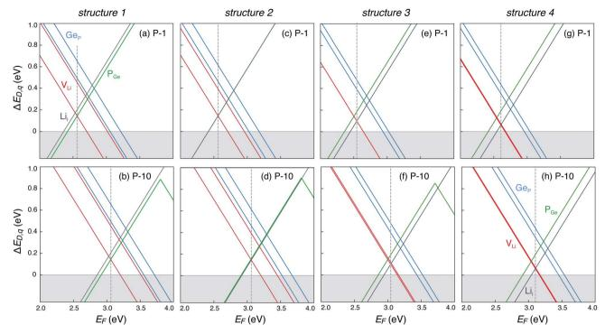
Fig. 5 Formation energies of native point defects ( $V_{Li}$ ,  $Li_i$ ,  $P_{Ge}$ , and  $Ge_P$ ) as functions of Fermi energy ( $E_F$ ) in LGPS structures 1–4 (Fig. 3) at elemental chemical potentials corresponding to P-1 (a, c, e and g), and P-10 (b, d, f and h).  $E_{\rm F}$  is referenced to the valence band maximum. Multiple lines of the same color represent the same defect type at different Wyckoff sites.
