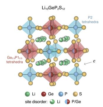
Fig. 1 Tetragonal crystal structure of  $\rm Li_{10}GeP_2S_{12}$  contains P2S<sub>4</sub> tetrahedra and ( $\rm Ge_{0.5}P1_{0.5}$ )S<sub>4</sub> tetrahedra with partially occupied Li sites in the c-axis channels and in the a-b plane bridging sites. The S sublattice and P2 sites are fully occupied.
