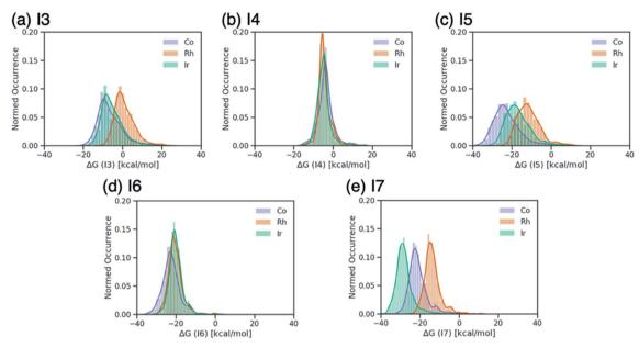
Fig. 2 Distributions of  $\Delta G$  values of intermediates (a) I3, (b) I4, (c) I5, (d) I6, and (e) I7 classified by metal center of the catalyst.  $\Delta G$  values are relative to  $\Delta G$ (I2).
