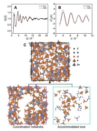
Fig. 3 Comparison of the experimental data (black lines) and the results of the RMC structural modelling (red lines) for 1. (A) X-ray total structure factor S(Q) and (B) EXAFS  $k^3\chi(k)$ . (C) The unit cell of the amorphous structure of 1 modelled by RMC. The coordination network and captured free dema and  $H_2PO_4^-/H_3PO_4$  are separately presented.
