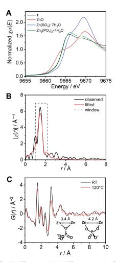
Fig. 2 (A) The XANES region of the XAFS spectra for the Zn<sup>2+</sup> K-edge of 1 (black) and references: ZnO (red), Zn(SO<sub>4</sub>)·7H<sub>2</sub>O (blue), and  $Zn_3(PO_4)_2 \cdot 4H_2O$  (green). (B) Radial distribution functions (RDF) of 1 (black line) and the fitting curve (red line). (C) The reduced pair distribution function (PDF) profile of 1 and Zn<sup>2+</sup>-Zn<sup>2+</sup> distances.
