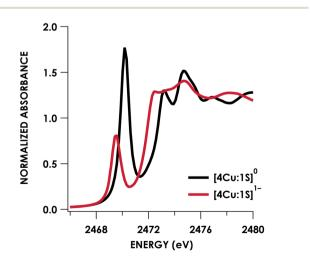
Fig. 4 S K-edge XAS data obtained for the  $[4\text{Cu}:1\text{S}]^{0/1-}$  redox couple. Pre-edge peaks corresponding to S 1s  $\rightarrow \psi^*$  excitations are located at 2470.2 eV for  $[4\text{Cu}:1\text{S}]^0$  and 2469.5 eV for  $[4\text{Cu}:1\text{S}]^{1-}$ .
