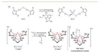
Scheme 1 Active participation of bridging sulfide ligands in  $N_2O$  activation by (a) binuclear and (b) and (c) tetranuclear synthetic copper sulfide models.
