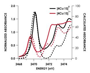
Fig. 6 Overlay of TDDFT-calculated (dashed) S K-edge XAS with experimental (solid) spectra obtained for the [4Cu:1S] $^{0/1-}$  redox series. TDDFT calculations were initiated from B3LYP single-point calculations with the CP(PPP) $^{34}$  basis set on Cu and the ZORA-def2-TZVP(-f) $^{38}$  basis set on all other atoms. Calculated spectra are shifted by +40.4 eV to correct for inaccurate core potential modeling endemic to standard hybrid DFT calculations.
