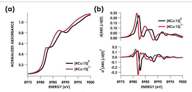
Fig. 3 (a) Cu K-edge XAS spectra obtained for the  $[4\text{Cu}:1\text{S}]^{0/1-}$  redox couple. (b) First (top) and second (bottom) derivative Cu K-edge XAS spectra. Isoenergetic pre-edge (1s  $\rightarrow$  3d) excitations are evident in the second-derivative spectra at 8979.8 eV. Rising edge inflection points occur at 8982.3 and 8985.9 eV for  $[4\text{Cu}:1\text{S}]^0$  and 8981.5 and 8984.8 eV for  $[4\text{Cu}:1\text{S}]^{1-}$ .
