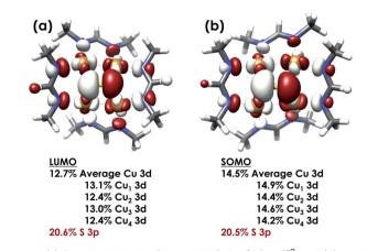
Fig. 5 (a) Restricted Kohn–Sham LUMO for [4Cu:1S]<sup>0</sup> and (b) quasi-restricted (QRO)<sup>33</sup> SOMO for [4Cu:1S]<sup>1—</sup>. Both MOs were calculated for truncated models using the B3LYP hybrid density functional with the CP(PPP) basis set on Cu and the scalar-relativistically recontracted ZORA-def2-TZVP(-f) basis set on all other atoms. Orbitals are plotted at an isovalue of 0.03 au.
